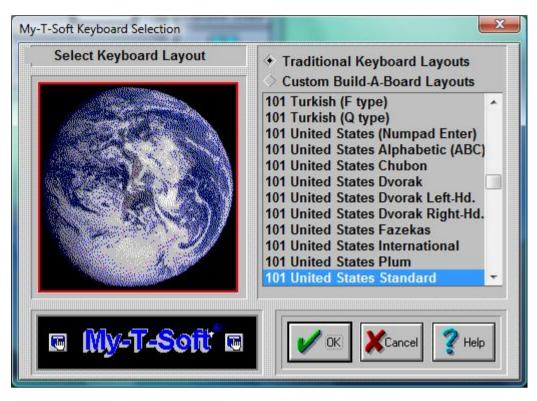
My-T-Soft can operate with many different keyboard layouts. By selecting the same keyboard layout that Windows uses, you can synchronize the display on My-T-Soft with the characters generated in your application.
